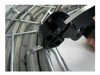
2. Slide the tail into the side entry and position the tool as shown. Position the tool against the base of the buckle.
