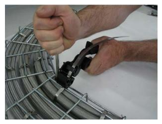
4. Maintain final handle pressure and rotate cutter bar upward for cut off.
