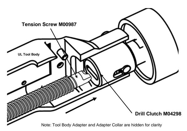
**Figure 3:** Align the end of the Tension Screw with the slot in the end of the Drill Clutch during assembly, as shown above.
