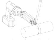
Do not force the tool against the clamp; it may result in a folded clamp tail.
