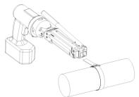
5. Actuate Drill until Tension Block is all the way forward against the tool body. Set Drill to clock-wise rotation. With cut-off handle down as shown, insert clamp tail into tool head slot. Actuate Drill until Drill's built-in clutch disengages. If Tension Block comes near its end of travel, release actuator switch and reverse Drill to pull more on clamp tail. Excessive use of disengaging Drill Clutch indicated by a loud ratcheting sound leads to premature wear of tension screw.
