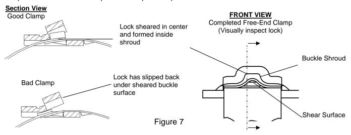
**Important:** Visually inspect lock formed in band as shown. If lock has slipped under the sheared surface of the buckle, remove clamp and install a new one at reduced tension by lowering the Drill Clutch torque setting.
