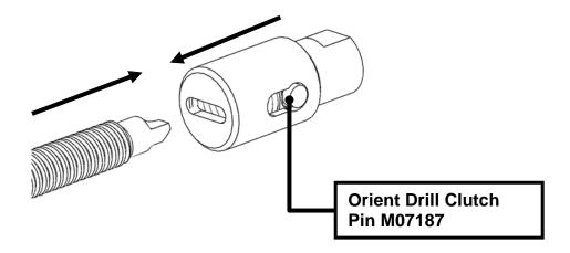
NOTE: Alignment is critical for proper tool function.
