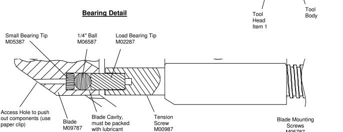
3. To gain access to bearing components: remove blade Mounting Screws (2 places) and slide Blade free. Paper clip may be used to push bearing components out of Blade. Wipe lubricant from components. If ball or bearing tips appears heavily worn, replace with new one. Note: 1/4" ball is made from hard tungsten carbide material, do not replace with regular ball bearing. (Smooth indention from ball in the bearing tips is normal).
