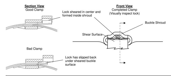
**Important:** Visually inspect lock formed in band as shown. If lock has slipped under the sheared surface of the buckle, remove clamp and install a new one at reduced tension by lowering the Drill Clutch torque setting.
