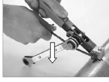
E) After the lock is secured, cut off the excess band tail by firmly pushing the cut-off handle downward.
