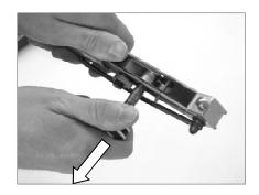
F) Carefully remove the excess band tail by removing the winding mandrel and ratchet from the tool body.
