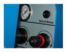
End-of-Stroke Indicates the desired clamp tension and cut-off has not occurred. Also shown is speed control with red lock ring.
