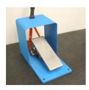
Dual function foot control valve. Pressing forward activates clamp installation. Heel action activates tail return and prepares for next clamp.
