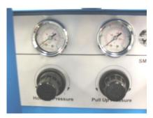
Air pressure setting can be made using the regulators and gauges on face of the tool.
