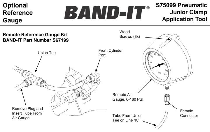
The Remote Reference Air Gauge will read air pressure in the front of the cylinder for both pull-up and holding pressures. To read gauge: When tensioning a clamp, the maximum pressure the gauge reads during the cycle is the pull-up pressure. After the tool switches over to the lower pressure holding cycle and before the clamp is rolled up in preparation for lock, the pressure shown is the holding pressure.
