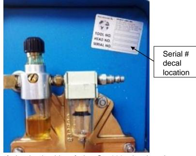
View of the back side of the S75099 showing the supplemental filtering and lubrication system as well as the  $\frac{1}{4}$ " N.P.T. air connection with typical quick connect coupling.
