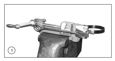
Place BAND-IT tool in vise. BAND-IT JR Adapter installs over nose of tool. Insert BAND-IT Junior or Junior SID Clamp in Tool and grip end of band by Band Gripper Lever contained in the slide block assembly of BAND-IT tool.
