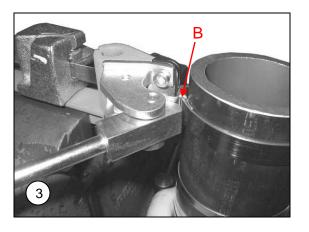
A. Roll hose over approximately 30°, BACKING OFF TENSION HANDLE ½ to 1 turn only through course of rollover, depending on type and size of hose.
