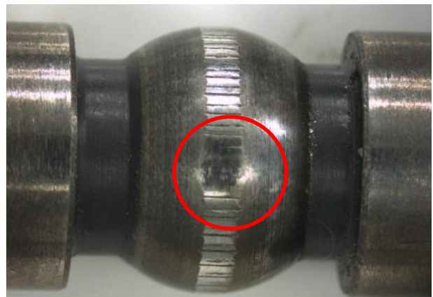
A worn out tension gripper: Ridges are worn off in some sections
