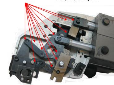
After the Maintenance Flip Cover is cleaned, lubricated, installed and Quick Release Pins are in place, apply tension to the Flip Cover Tightening Screw and Flip Cover Head Screws. Refer to pages 7, 17.
