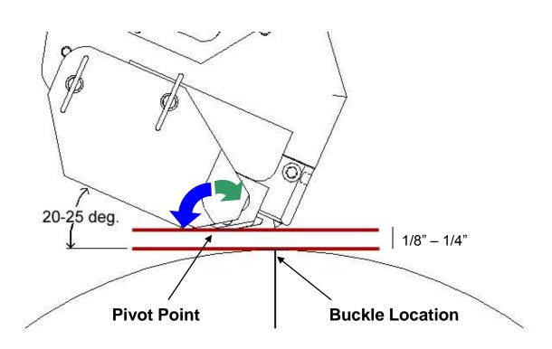
As the band is tensioning, the tool may rotate clockwise up to 5 degrees about the pivot point (Green Arrow). During the cut-off cycle, the tool must be allowed to rotate counterclockwise up to 35 degrees (Blue Arrow). Because of this movement, **BAND-IT** recommends that the tool be mounted in a fixture that will provide adequate rotation during both cycles.
