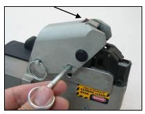
1. Loosen the Flip Cover Tightening Screw and Flip Cover Head Screws (see note above) to remove both Quick Release Pins as shown.
