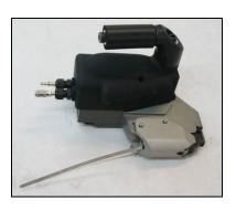
5. After clamp is completed, clamp tail scrap must be removed from tool. Clamp tail scrap is not ejected automatically. Tool is now ready for next clamp.
