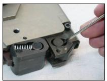
4. When installing the Cutter Blade Pin, use a small screwdriver to push the front gripper toward the back of the tool.
