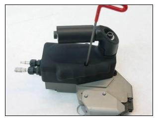
The Timing Valve will be affected over time by contaminants in the air system. Moisture, dirt particles, oil and solvents can cause blockage or fluctuations in the tool performance.
