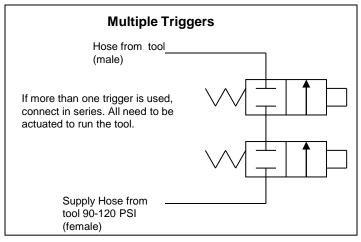
Connect the 2 hoses extending from the tool to the ports of the valve. As the hoses are not marked, they may need to have their connection on the valve reversed if the remote trigger does not start the tool.
