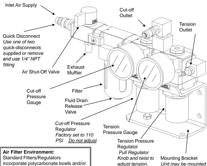
incorporate polycarbonate bowls and/or observation windows. DO NOT use in an environment that will expose the above mentioned components to synthetic fluids, organic solvents, chemicals, cutting lubricants, thread lock solutions or similar materials.
