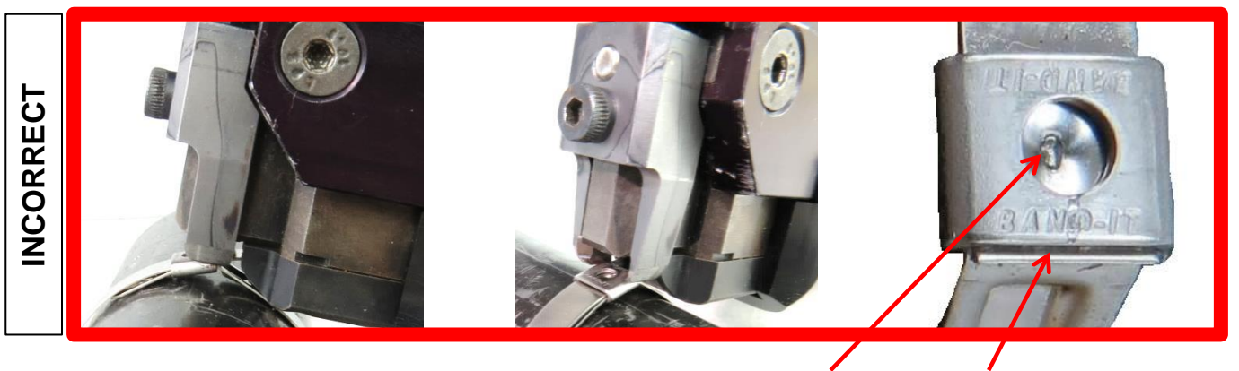
Incorrect alignment results in shallow dimple & excess tail
