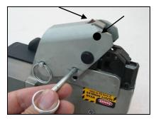
1. Loosen the Flip Cover Tightening Screw and Head Screws (see note above) to remove both Quick Release Pins as shown.
