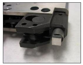
Once the pin is removed, grasp the Knife Assembly with a pair of needle-nose pliers and pull out of tool head. Examine for wear and rotate or replace if needed.
