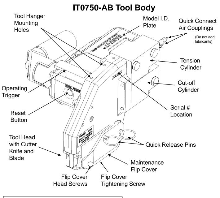
*Important:* Before disassembling tool, be sure to shut-off air supply on the Air Controller Module.
