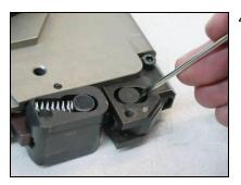
4. When installing the Cutter Blade Pin, use a small screwdriver to push the front gripper toward the back of the tool.
