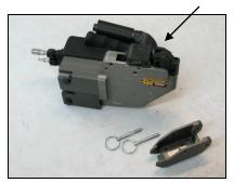
2. Remove Flip Cover and Tension Block Assembly for cleaning and lubrication.
