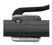
1. Remove gripper. Align gripper pin hole with notch in tool frame. Using a punch and hammer, punch pin out of slide block.
