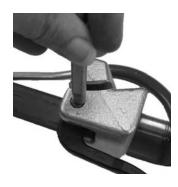
3. Replace pin. Gripper spring must be seated in tension screw hole. Align gripper hole with slide block hole, insert pin in hole and hammer pin in place.
