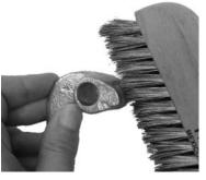
2. Using a wire brush, clean any foreign matter from teeth of new gripper.
