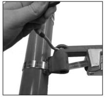
6. Pull cutting handle to cut the band. When applying Giant Band clamps, prior to cutting off clamp, release band gripper and push tool nose away from buckle approx. ¼".
