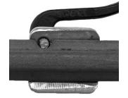
1. Remove gripper. Align gripper pin hole with notch in tool frame. Using a punch and hammer, punch pin out of slide block.
