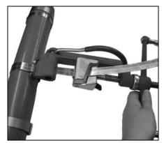
5. Roll tool over buckle, backing off with tension handle1- 1½ turns throughout entire rolling operation. Failure to back off tension with tension handle throughout entire course of roll-over may result in breaking of band. There is no loss of tension as band released is used up in the bend.
