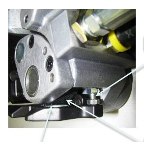
Reversible Slide plate. Only replace with **BAND-IT** part number XE4819 Gripper gap adjustment screw and lock nut
